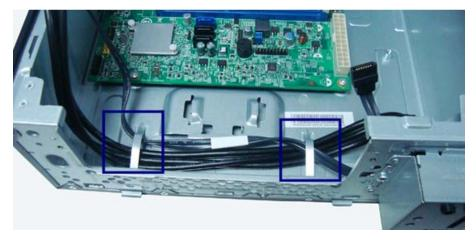
3. Disconnect the front I/O and optional card reader from their mainboard connectors.
